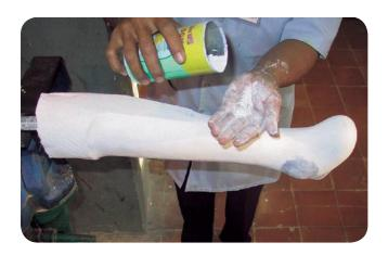
Heat the EVA cone in an oven for about 5 minutes at 120°C and then pull it over the plaster positive.
