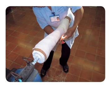
▶ Trim the distal section of the EVA cone with a knife and smooth it by grinding.
