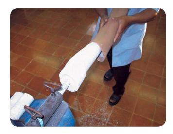
▶ To keep the EVA foam in the same shape as the plaster positive, secure it with elastic bandages or place it under vacuum until it has cooled down.
