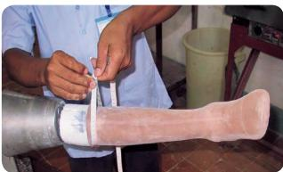
Before draping the polypropylene, pull a nylon stocking over the soft socket and dust it with talcum powder.
