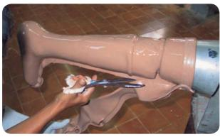
Keep the vacuum on for about 5 min., but wait until the PP has completely cooled down before removing the mould from the vacuum cone.
