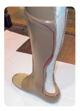
To avoid damaging the EVA foam, do not cut the forefoot opening with an oscillating saw or knife. Instead, carefully grind it off.
