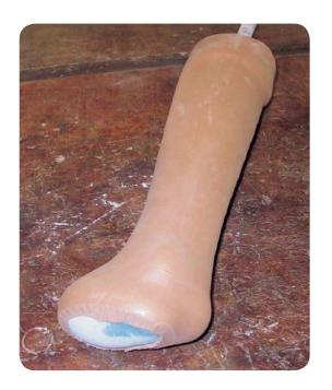
Apply two layers of Neoprene contact glue to the trimmed section and to the 12 mm EVA foam socket cap.
