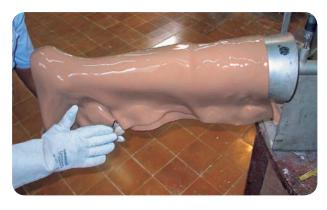
▶ With scissors or a knife, cut off the excess along the welding seam while the PP is still hot.
