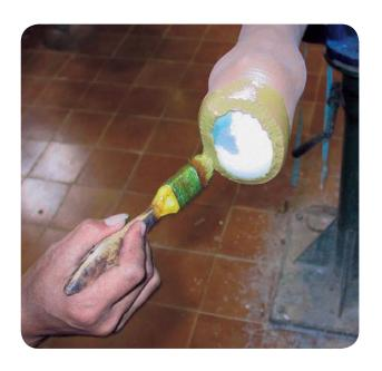
▶ Heat the cap for 2 to 3 minutes at 120°C in an oven and glue it onto the soft socket.
