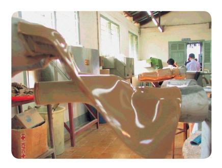
Drape the polypropylene over the plaster model and stick the sides together along the medial side of the socket. Tighten the polypropylene around the suction cone or tube using a bicycle inner tube, rope or stocking, then open the vacuum valve.
