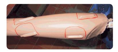
When the polypropylene has cooled, mark the trim lines of the hook cable attachments and cut with an oscillating saw.
