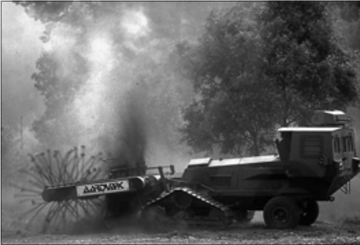
A military minefield breaching vehicle can use flails to open a path for advancing forces. However, their clearance rate is inadequate for humanitarian clearance operations, which must achieve a clearance rate of 99.6%.
