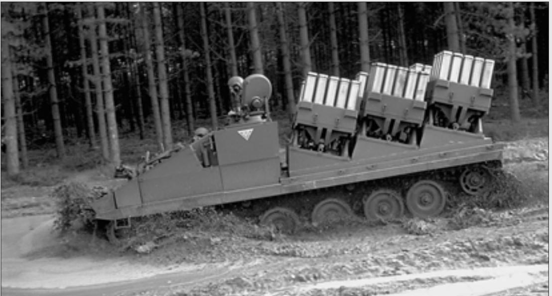
Launching system for scatterable antipersonnel mines: more than a thousand mines can be spread over a large area within a few minutes © The Military Picture Library photo T. Simpson
