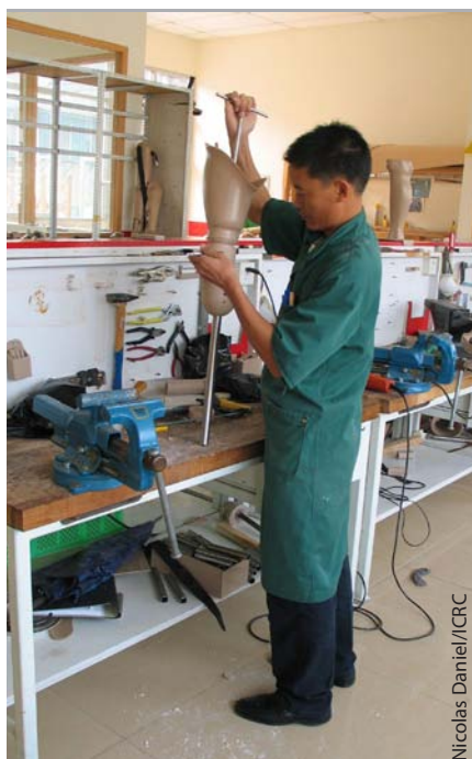
A bench technician aligns a trans-femoral prosthesis at the centre's orthopaedic workshop
