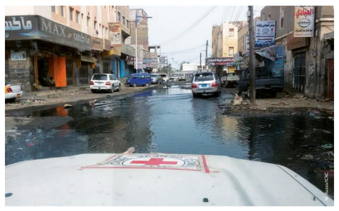
**Photo 6.** Interconnectivity between essential services needs to be understood and properly integrated into an emergency response to a breakdown in order to avoid counterproductive effects. Retrofitting the broken water supply network to this quarter without addressing the damaged sewage evacuation network would increase the exposure of the population to public health risks by causing sewage to spill over into the streets. (Aden. 2015)
