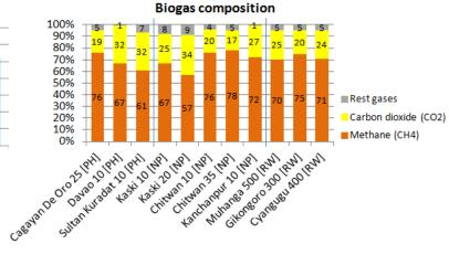
Figure 4: Comparison of daily biogas productionFigure 5: Comparison of biogas composition in AD systems of Philippinesper person[PH], Nepal [NP] and Rwanda [RW]
