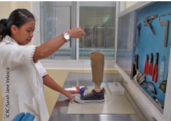
At DJF's new workshop, orthopaedic technologist Glorycel Lasquite checks a prosthetic device made of polypropylene for correct balance.
