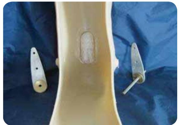
Put both joints back in place; fix them with foot shell bolts and position properly to mark the rivet holes.
