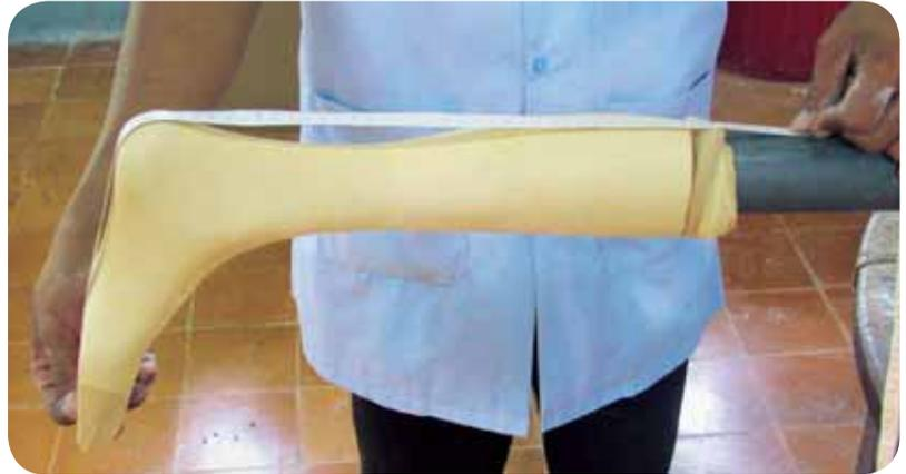
Heat the polypropylene at 180° for 20 to 25 minutes, depending on the thickness of the polypropylene and the efficiency of the oven.
