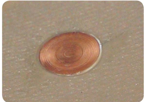
Insert the rivet, head inside, and install the washer outside.
