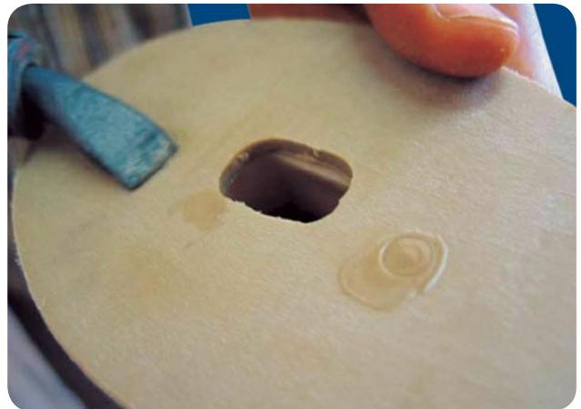
Attach the concave cylinder (with the opening in front) to the foot and the convex ankle.
