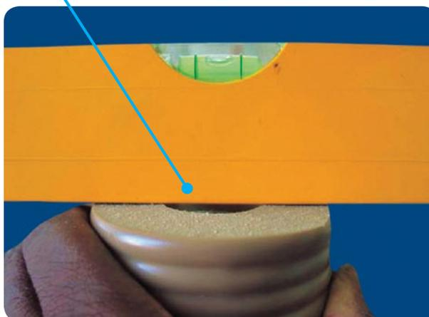
For maximum strength, keep a minimum PP thickness of 2 to 3 mm under the cup.
