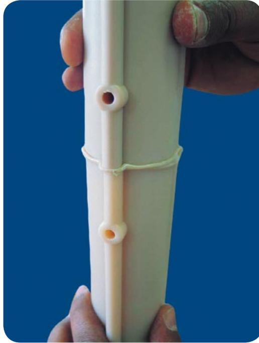
Concave cylinders correctly welded
