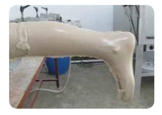
Carefully file the PP over the bushings down to the level of the bushings, as shown. These surfaces have to be flat and parallel.
