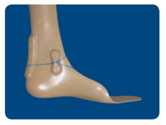
▶ For AFO <u>with free plantar flexion</u>, draw a "V" posterior to the midline of each cavity. Ensure that the "V" does not extend forward past the centre of the cavity.
