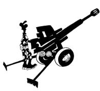
**Howitzers.** These are light, manoeuvrable weapons with a calibre of between 76 mm and 105 mm. Howitzers can fire at ranges up to 13 km.
