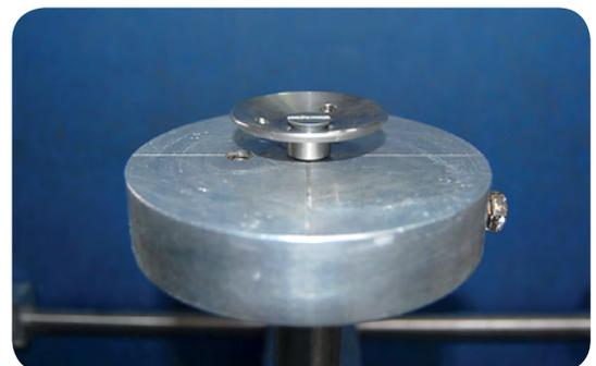
Use a standard alignment jig to make certain that the heavy-duty nut is properly aligned
