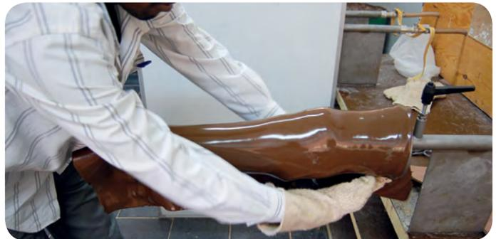
Add 10 mm of hot PP (square shapes of the same width as the mould)
