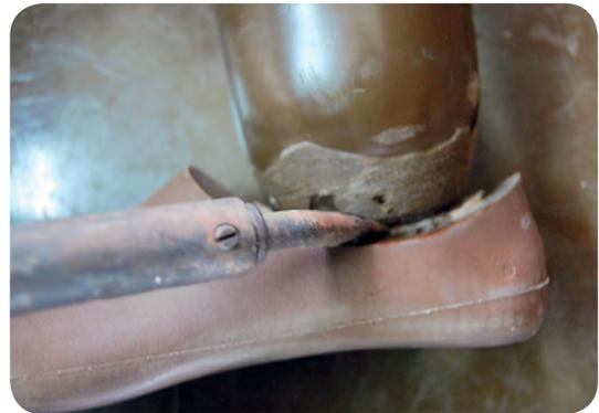
Weld the components with the PP rod so that the foot is firmly attached to the socket
