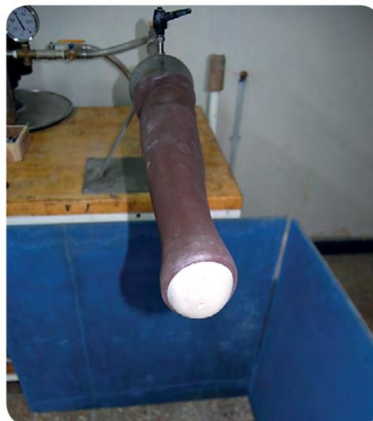
Apply contact adhesive to the skived edges of the distal end and prepare a cap (for the distal end)
