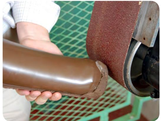
**Machine the distal end to reveal the countersunk screw**
