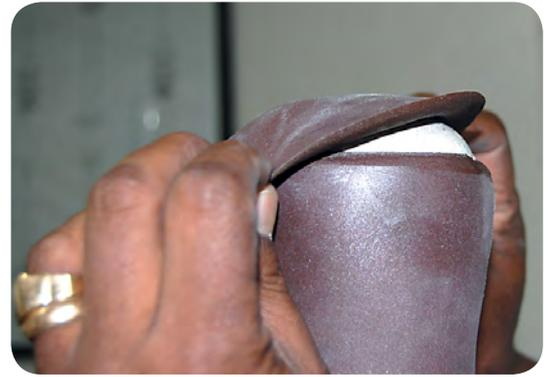
Grind the excess EVA to produce a smooth finish
