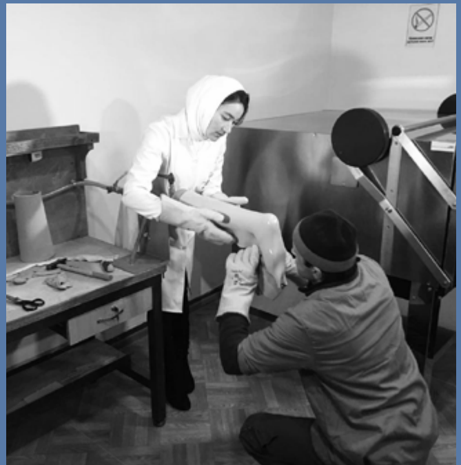
Juraeva Nigora, one of the MoveAbility sponsored female students at the VIETCOT, who is working in Khujand branch after graduating as orthotist. On the right bottom of the picture is one of the bench workers assisting her by thermoforming of an orthosis. Picture was taken in the newly opened workshop.
