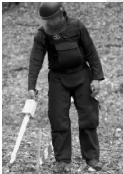
A battle area clearance expert testing his "fluxgate magnetometer" detector before beginning to search for unexploded cluster bomblets.
